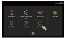
Step 3: Enter the countdown prompt, "Please confirm whether to shut down", click "OK" to enter the soft shutdown state, click "Return" to cancel the operation, in the soft shutdown state, the screen turns off, and the lighting system is still on. (Long press the screen for 3 seconds to restart the machine in soft shutdown state)
