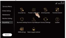
Step 6: Select "Left grinder", click the "Run" button, the powder will fall into the grounds box, and wait for the coffee machine to finish working;
