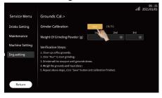
Step 6: Open the door of the coffee machine, take out the grounds container, weigh the coffee powder in the grounds container and record it in the machine;
